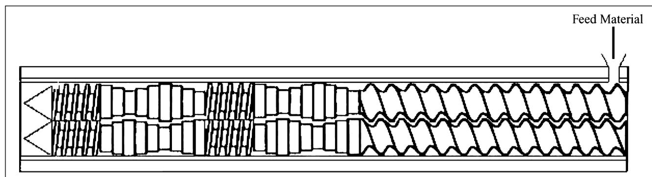
**Figure 1 – Schematic representation of screw configuration.**
