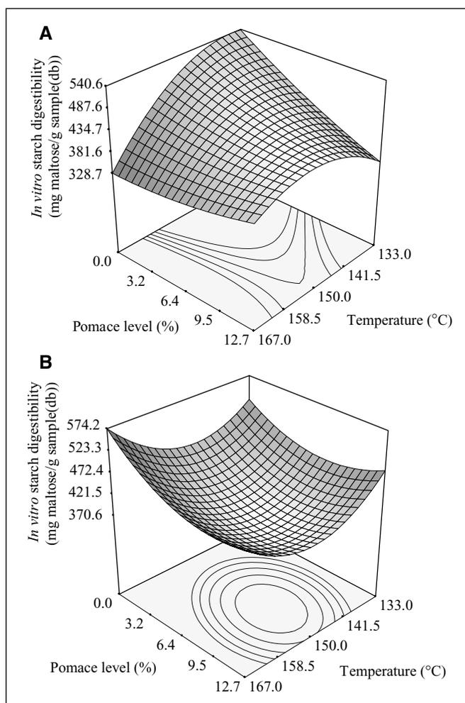
**Figure 7 – Response surface plot for the effect of temperature and pomace level on the *in vitro* starch digestibility of (A) barley–tomato pomace extrudates, (B) barley–grape pomace extrudates at screw speed of 175 rpm.**
