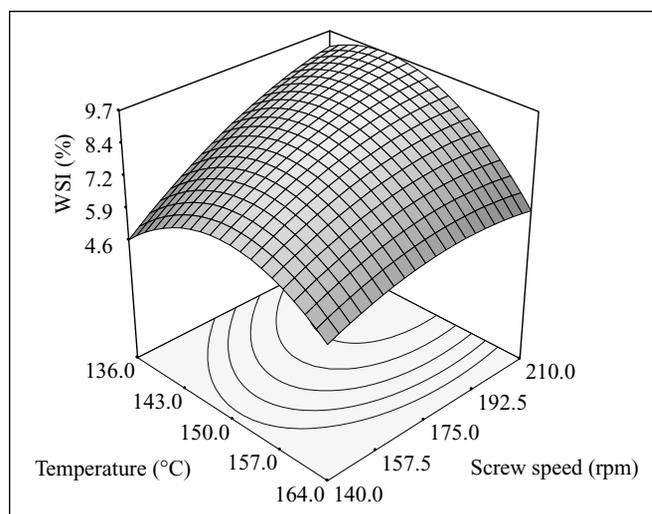
**Figure 3—Response surface plot for the effect of screw speed and temperature on WSI of barley extrudates.**
