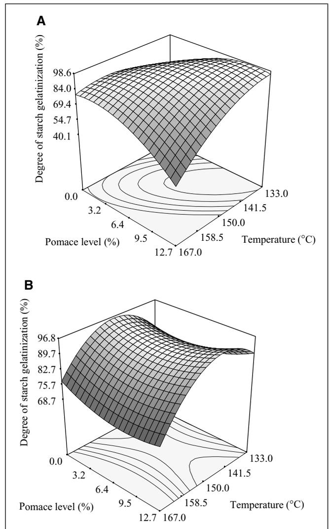
**Figure 5—Response surface plot for the effect of temperature and pomace level on the degree of starch gelatinization of (A) barley-tomato pomace extrudates, (B) barley-grape pomace extrudates at screw speed of 175 rpm.**
