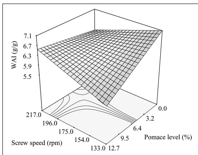
**Figure 2—Response surface plot for the effect of pomace level and screw speed on WAI of barley-grape pomace extrudates at a temperature of 150 °C.**
