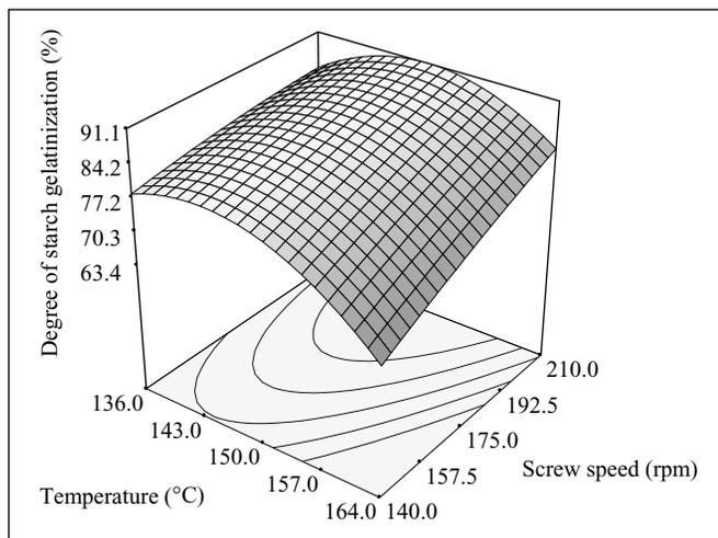
**Figure 4—Response surface plot for the effect of screw speed and temperature on the degree of starch gelatinization (%) of barley flour extrudates.**
