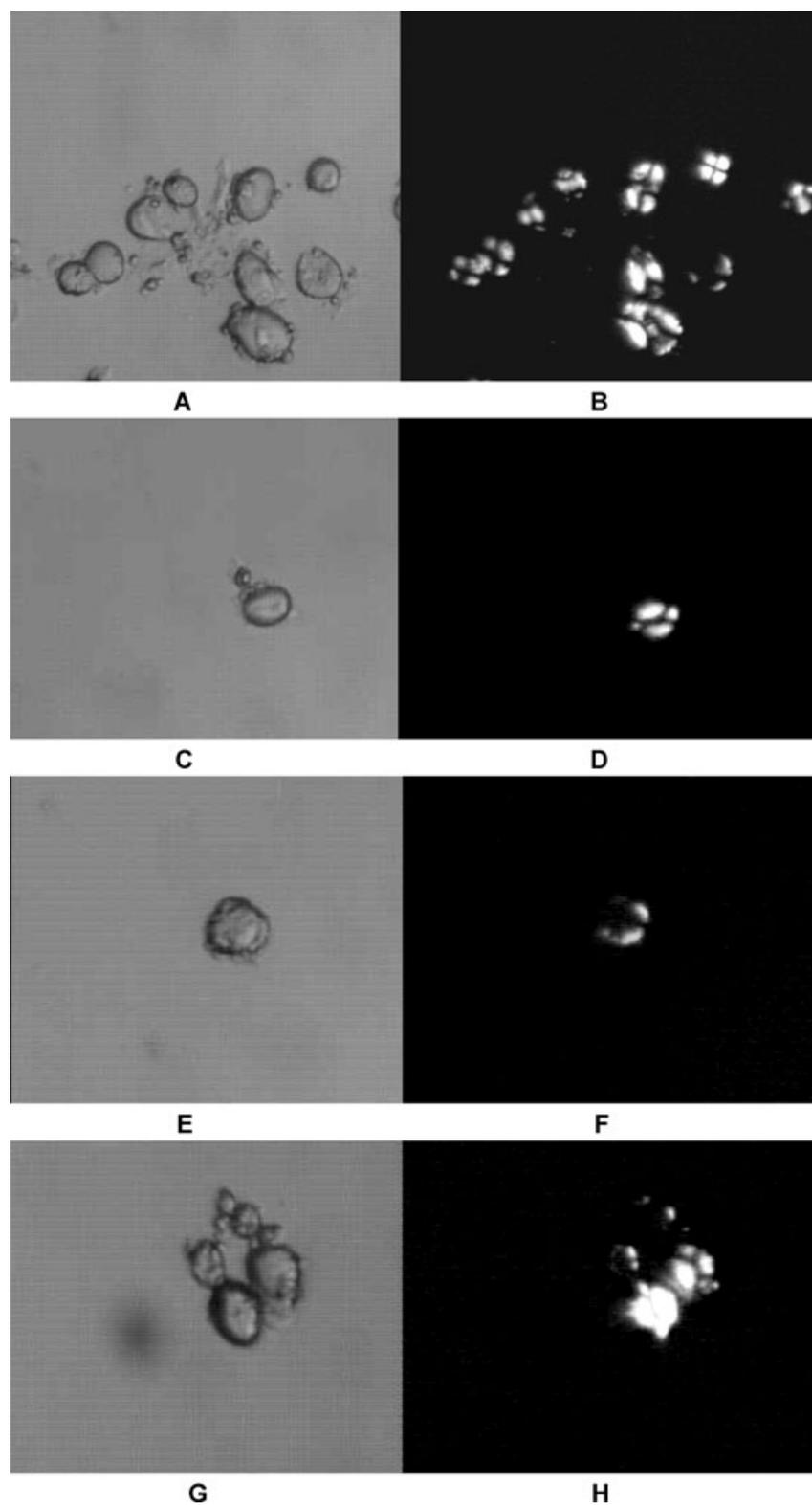
**Figure 6**— Images of barley flour under bright field (A) and polarized light (B); barley extrudate produced at 164 °C and 175 rpm screw speed under bright field (C) and polarized light (D); barley–tomato pomace extrudate produced at 160 °C, 150 rpm screw speed, and 2% tomato pomace under bright field (E) and polarized light (F); barley–grape pomace extrudate produced at 167 °C, 175 rpm screw speed, and 6% grape pomace under bright field (G) and polarized light (H).
