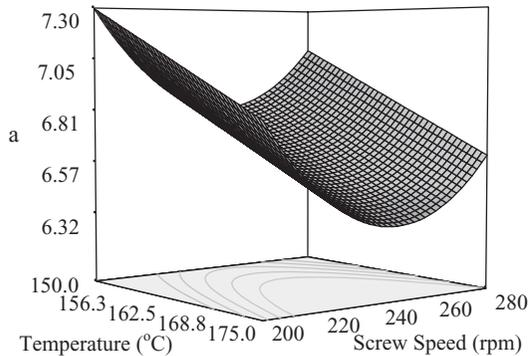
FIG. 7. RESPONSE SURFACE PLOT FOR THE REDNESS (*a*) VALUE AS A FUNCTION OF TEMPERATURE AND SCREW SPEED AT 18% DURUM CLEAR FLOUR, 7% PARTIALLY DEFATTED HAZELNUT FLOUR, 5% FRUIT WASTE CONTENTS AND 12% MOISTURE CONTENT
