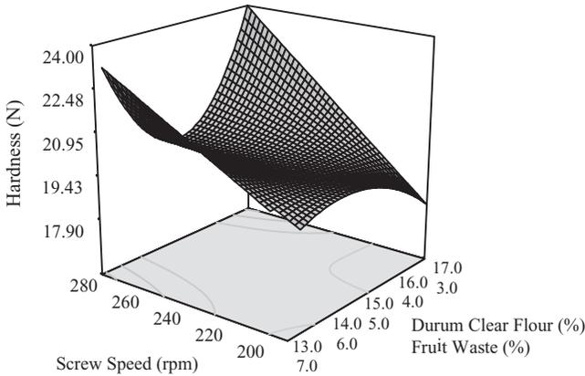
FIG. 4. RESPONSE SURFACE PLOT FOR HARDNESS AS A FUNCTION OF SCREW SPEED, DURUM CLEAR FLOUR AND FRUIT WASTE CONTENT AT 12% MOISTURE CONTENT, 10% PDHF CONTENT AND 150C BARREL TEMPERATURE
