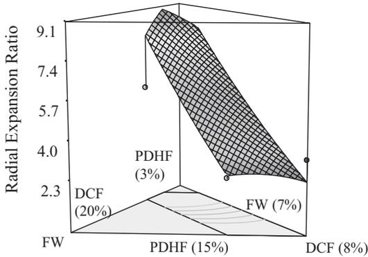
FIG. 1. RESPONSE SURFACE PLOT FOR RADIAL EXPANSION RATIO AS A FUNCTION OF COMPONENTS AT 12% MOISTURE CONTENT, 200-rpm SCREW SPEED AND 150C BARREL TEMPERATURE
