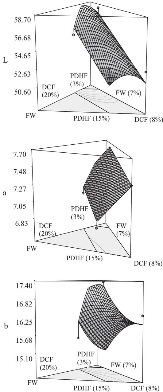
FIG. 5. RESPONSE SURFACE PLOT FOR COLOR VALUES (lightness [L], redness [a] and yellowness [b]) AS A FUNCTION OF COMPONENTS AT 12% MOISTURE CONTENT, 200-rpm SCREW SPEED AND 150C BARREL TEMPERATURE
