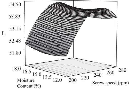
FIG. 6. RESPONSE SURFACE PLOT FOR THE LIGHTNESS ( $L$ ) VALUE AS A FUNCTION OF MOISTURE CONTENT AND SCREW SPEED AT 13.5% DURUM CLEAR FLOUR, 13.5% PARTIALLY DEFATTED HAZELNUT FLOUR, 3% FRUIT WASTE CONTENT AND BARREL TEMPERATURE OF 150C
