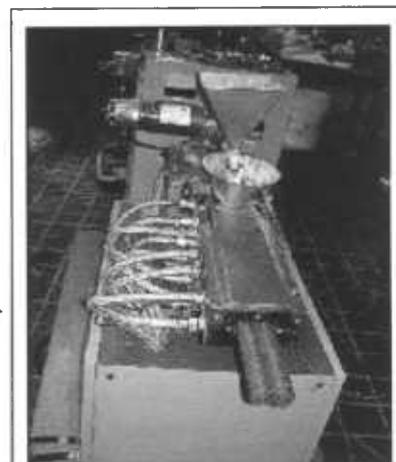
Figure 1. Twin-Screw Extruder
