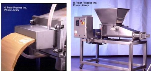
Extrusions can be done through heating or cooling dies to enhance surface texture.
