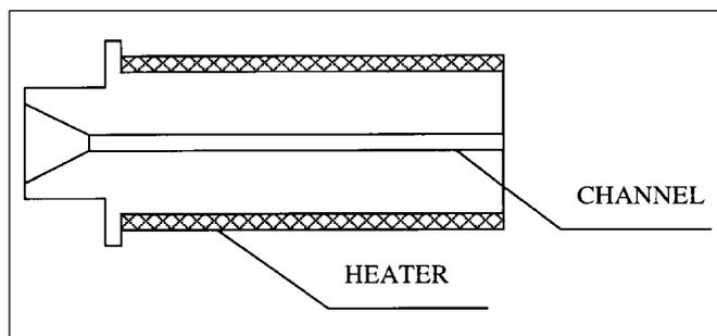
Fig. 1—A simplified diagram of the extruder die.
