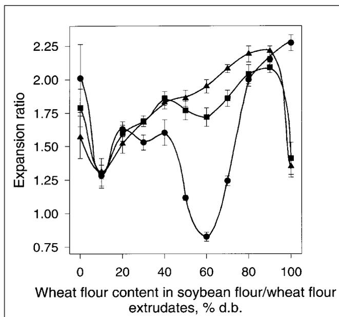
**Fig. 3—Expansion ratio of extrudates as related to wheat flour content in extruded soybean flour/wheat flour blends. ● 16%, ■ 17%, ▲ 18% w.b. of moisture content in the extruded blends.**
