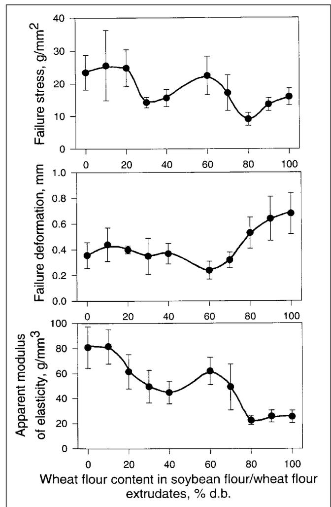
**Fig. 4—Failure stress, failure deformation and apparent elasticity modulus of extrudates as related to wheat flour content in extruded soybean flour/wheat flour blends.**
