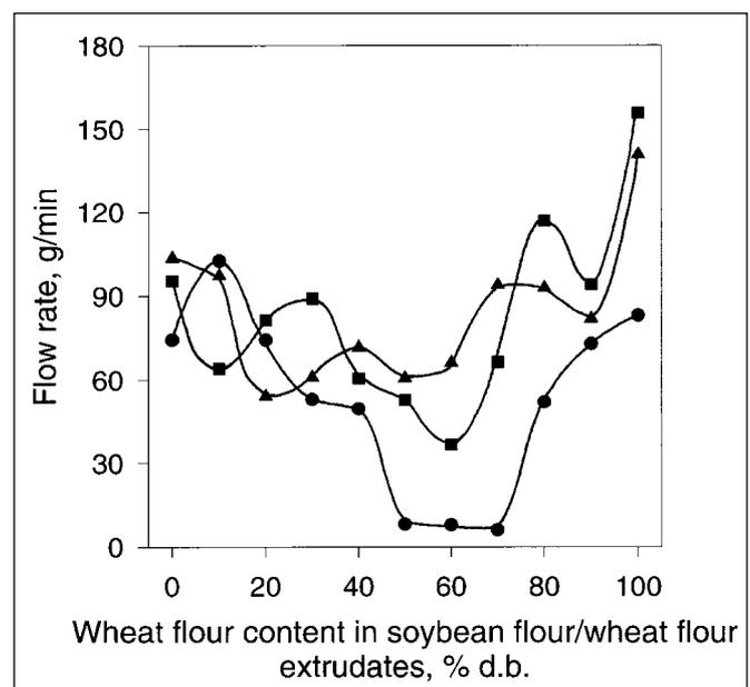
Fig. 2—Flow rate at the die exit as related to wheat flour content in extruded soybean flour/wheat flour blends. ● 16%, ■ 17%, ▲ 18% w.b. of moisture content in extruded blends.
