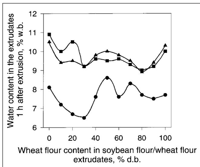
**Fig. 5—Moisture content in extrudates 1 h after extrusion as related to wheat flour content in extruded soybean flour/wheat flour blends. ● 16%, ■ 17%, ▲ 18% w.b. of moisture content in the extruded blends.**
