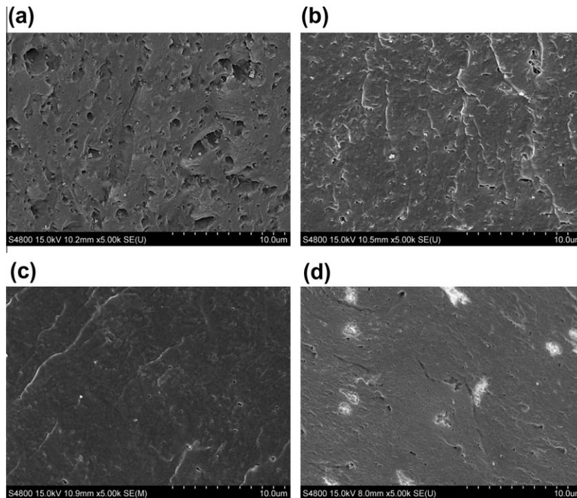
Fig. 6. SEM micrographs taken at the break surface of SPI-based products fractured in liquid nitrogen: (a) SPI20, (b) SPI-GE, (c) SUC30 and (d) LAC30.
