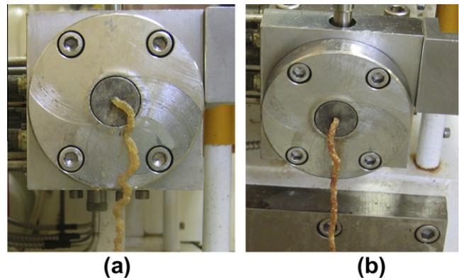
Fig. 2. Products obtained at the extruder die for (a) SPI with sucrose and (b) SPI with lactose.
