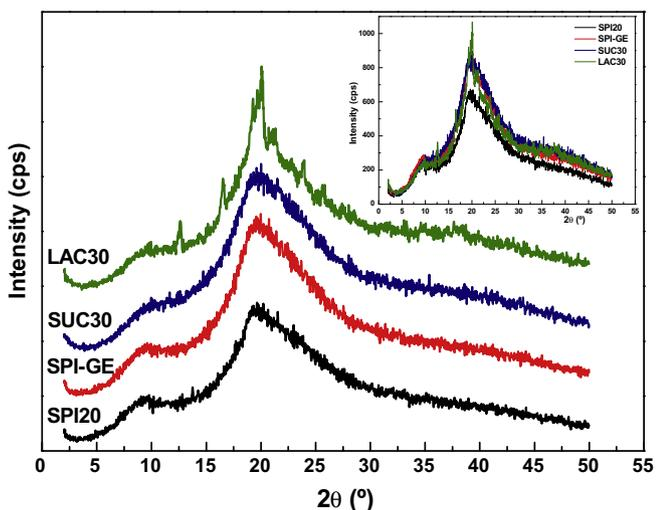
Fig. 4. XRD patterns for SPI-based products with different additives.
