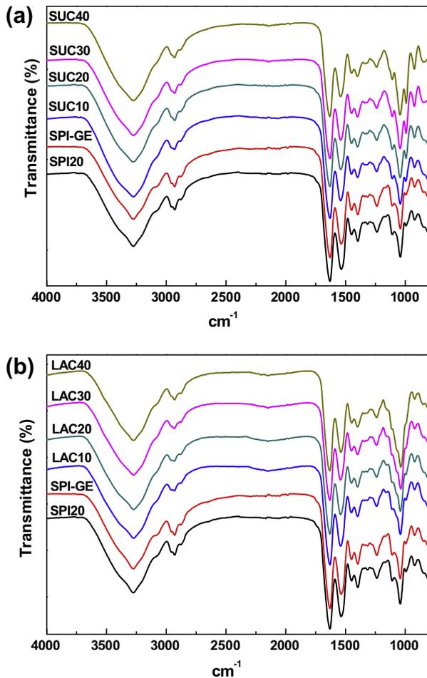
Fig. 5. FTIR spectra of SPI-based products with different contents of (a) sucrose and (b) lactose.
