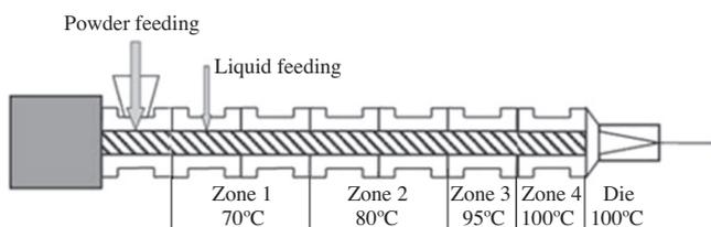
Fig. 1. Schematic diagram of the twin-screw extruder employed in this study.
