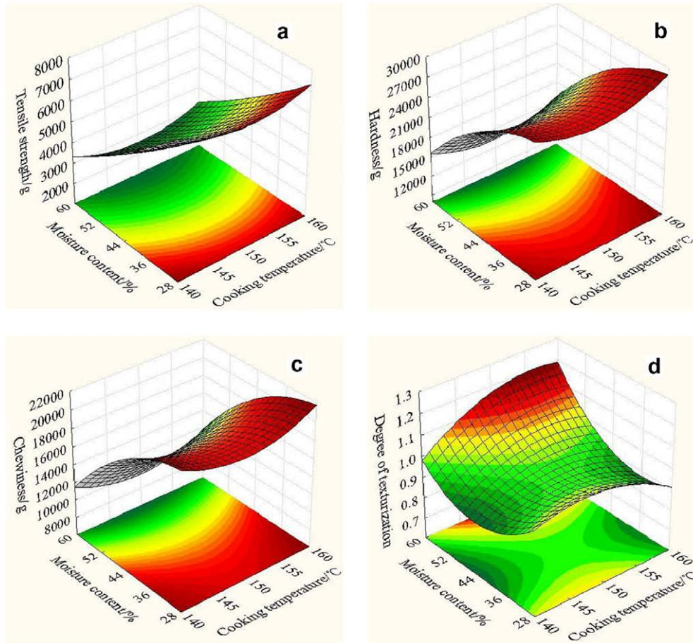
**Fig. 4.** Tensile strength (a), hardness (b), chewiness (c) and degree of texturization (d) versus moisture content and cooking temperature with screw speed 160 rpm and feed speed 20 g/min.
