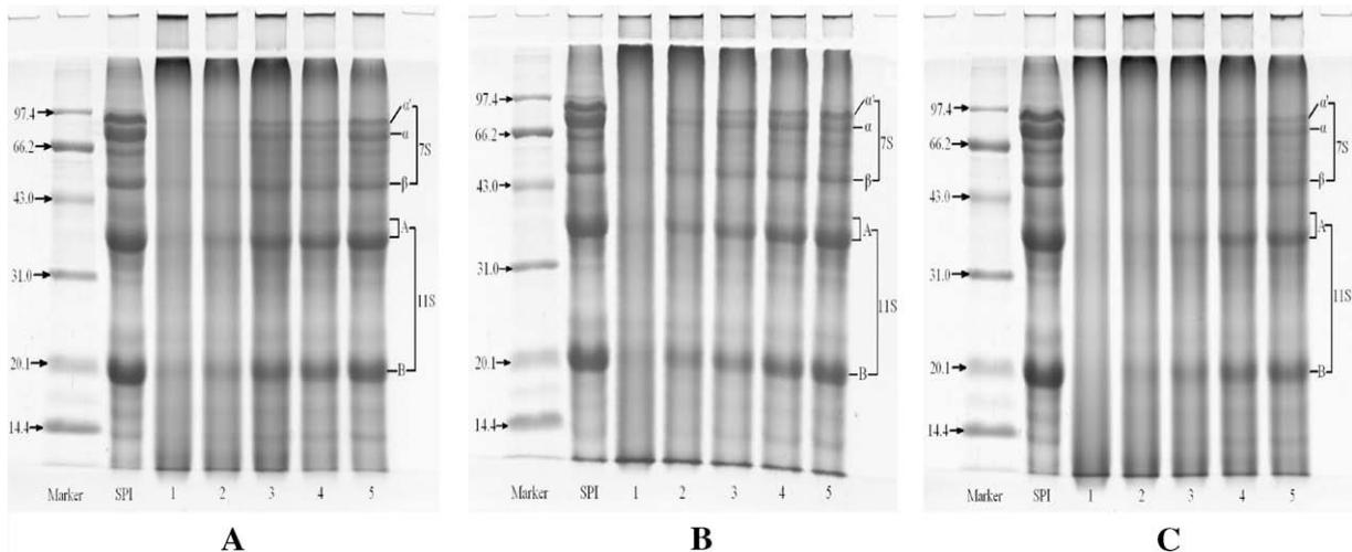
**Fig. 5.** Vertical SDS-PAGE of samples extruded at (A) 140 °C, (B) 150 °C and (C) 160 °C (1–5 indicates 28%, 36%, 44%, 52% and 60% moisture content, respectively).
