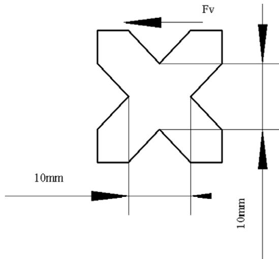
Fig. 2. Sampling sketch for degree of texturization test.
