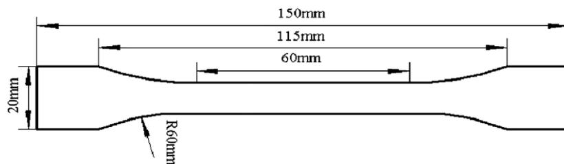
Fig. 1. Sampling sketch for tensile strength test.
