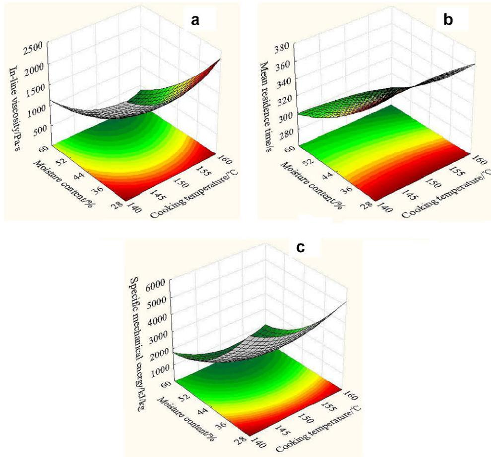
Fig. 3. In-line viscosity (a), mean residence time (b) and SME (c) versus moisture content and cooking temperature with screw speed 160 rpm and feed speed 20 g/min.
