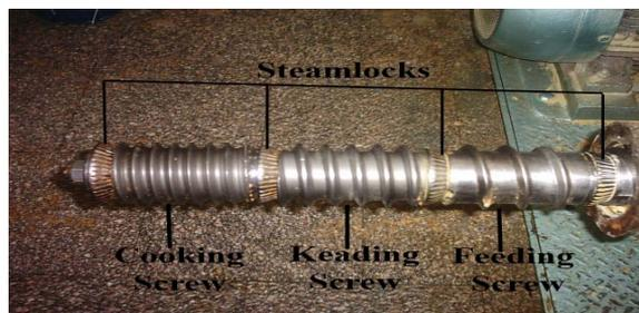
**Fig. (10): A photo for the extruder's screw including the three screw zones and the four steamlocks after development**
