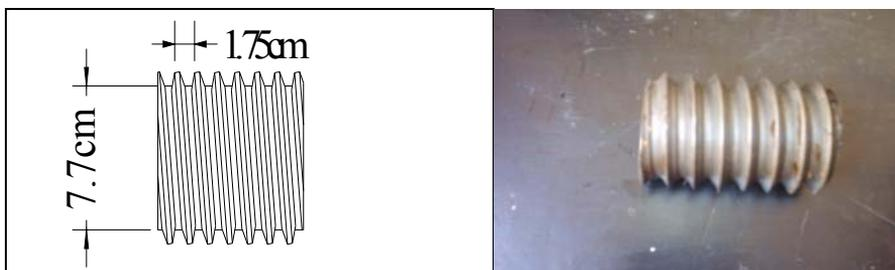
**Fig. (8): The design of final screw design.**
