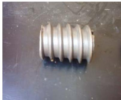
**Fig.(7): A photo of the new kneading screw part.**
