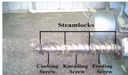
**Fig. (2): A photo for the extruder's screw including the three screw sections and the four steamlocks.**
