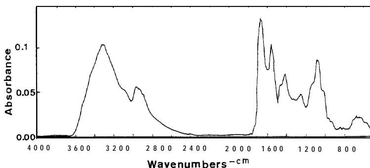
Fig. 5. The subtraction spectrum deducted the FT-IR spectrum of products from that of raw material. Absorbance of carbonyl at  $1750\text{-cm}^{-1}$  was used as a standard mark on the computer calculation.
