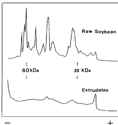
Fig. 6. Denstogram of raw materials and extrudate. The SDS-polyacrylamide gel electrophoresis was done by the method of Weber and Osbom, with 12% acrylamide gel concentration and 25  $\mu$ g of protein put on each gel. Current was 20 mA.
