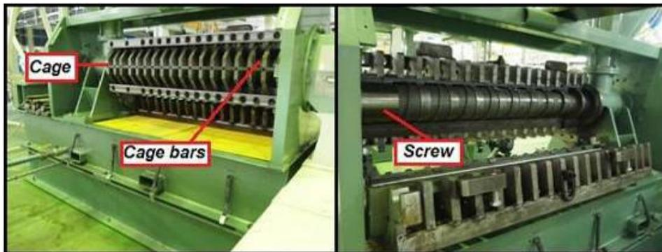
There are other ways to expand oil processing as well. Extrusion may be able to increase press efficiency and yields by allowing oil cells to rupture, making the oil easier to access and remove. A great example of this is the **Insta-Pro ExPress® process**. In the case of soybeans, this process is able to extract up to 66% of the available oil out of the seed.
