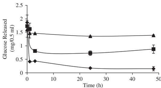
**Fig. 3.** Effect of saccharification temperature on Accellerase activity. Diamond: 65 °C; rectangle: 50 °C; triangle: 45 °C.
