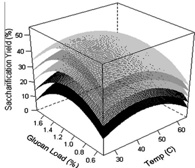
**Fig. 4.** Effect of glucan load, temperature and enzyme loading on saccharification yield of EAEP extruded FFSF fiber fraction after 27 h incubation. Enzyme loads (FPU/g-glucan) from bottom to top: 6.5 (black); 53.8 (black and grey); 101.1 (grey); 148.4 (dark grey); 196.0 (light grey).
