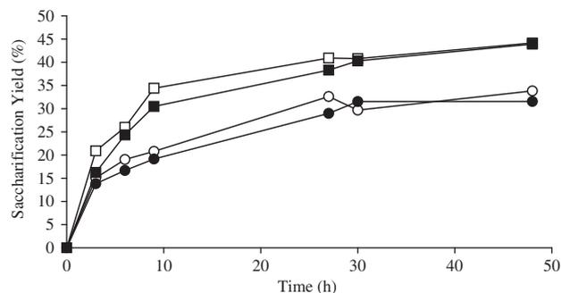
**Fig. 2.** Effect of extrusion and presence of protease during the extraction on saccharification yield, White circles: AEP FFSF; black circles: EAEP FFSF; white rectangles: AEP extruded FFSF; black rectangles: EAEP extruded FFSF. LSD = 8.34.
